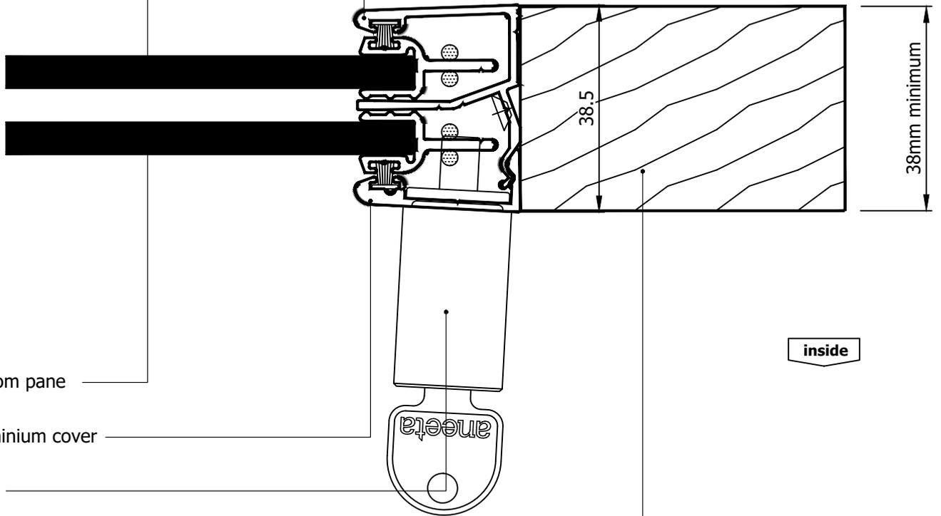
Aneeta inserts suit a variety of manufacturers door types. It is recommended to use at least a 190mm bottom rail and mortised corner joints. (to limit door movement)
