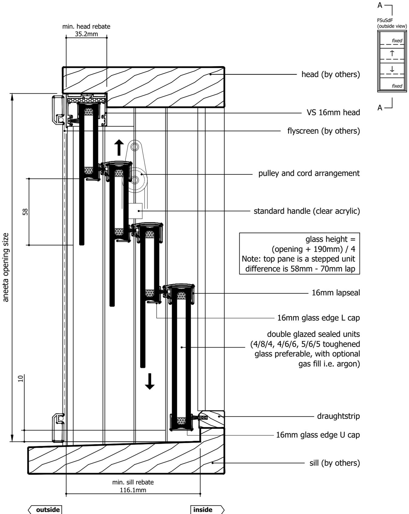
M:\Documentation\Website Downloads\3. Timber Frames\1. Vertical\1. Double Hung\VS 4P16C FSuSdF T (G) - 4 pane 16mm double glazed CLEARSTEP sashless vertical sliders in timber frames FSuSdF.dwg
